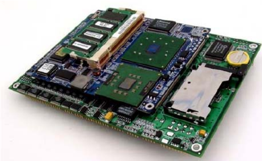
EPIC form-factor Custom Application Baseboard with ETX COM installed on top
