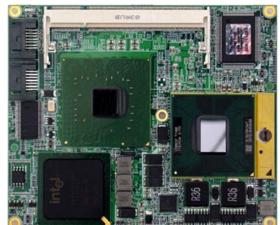
ETX-945-T7400 COM with Core2Duo CPU
